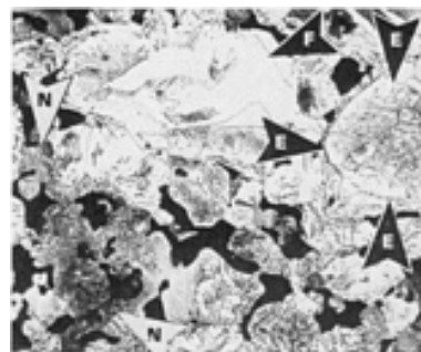
Fig. 99 Diffusion-alloyed steel (Fe-1.75Ni-0.5Mo-1.5Cu-0.5C, 6.7 g/cm 3 ), pressed at 410 to 480 MPa (60 to 70 ksi) and sintered 30 min at 1120 °C (2050 °F) in dissociated ammonia. Arrows N show nickel-rich regions containing martensite or bainite platelets; arrows E, a eutectoid colony with a white diffusion layer on the periphery. Arrow F indicates ferrite. 2% nital. 330×
