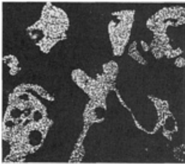
Fig. 158 M2 tool steel, water-atomized, vacuum-annealed powder. Irregular particles with a fine carbide phase. Equal parts 4% picral and 4% nital. 645×
