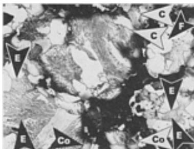
Fig. 63 Atomet 28 iron powder with 2% Cu and 0.5% C ( 6.7 \text{ g/cm}^3 with 275 MPa, or 40 ksi, minimum yield strength). See Fig. 53 for processing. Arrows E show eutectoid (pearlite); arrow F, white ferrite grains. Arrows C indicate isolated or divorced eutectoid in the form of separate \text{Fe}_3\text{C} platelets. Arrows Co show coring from copper dissolving in the outer regions of iron particles. 2% nital. 310×
