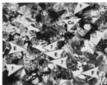
Fig. 90 Same as Fig. 88, but etched. The 2% Cu causes the nickel to dissolve, eliminating the nickel-rich regions. Arrows ? surround regions where the nickel probably was. These regions are darkened by the coring caused by copper dissolving there and contain carbide platelets. Another cored region is marked Co. Arrows E mark unresolved eutectoid, and arrow F indicates a white ferrite grain. 2% nital. 310×
