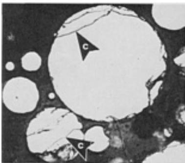
Fig. 159 Fe-31Si, water-atomized master-alloy powder (-100 mesh). Regular particle shape implies low green strength. Particles cracked (arrows C) during processing. As-polished. 645×
