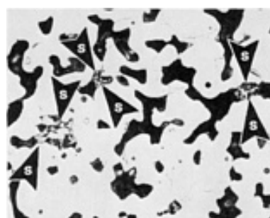
Fig. 85 Carbon-reduced sponge iron powder with 0.5% S blended as elemental fines. See Fig. 81 for processing ( 6.4 \text{ g/cm}^3 with 103 MPa, or 15 ksi, minimum yield strength). Arrows S show two-phase sulfide mixtures of MnS and FeS, which lie within the pores. 2% nital. 330\times
