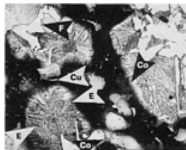
Fig. 65 Same as Fig. 63, but with 5% Cu and 0.5% C ( 6.7 \text{ g/cm}^3 with 344 MPa, or 50 ksi, minimum yield strength). At 5% Cu, some residual copper-rich phase is shown as thin, light-colored slivers (arrow Cu). Arrows Co show bands of coring from copper diffusion into the iron. Arrows E indicate eutectoid (pearlite). Arrow F shows ferrite grain. 2% nital. 330×
