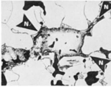
Fig. 91 Nickel steel (atomized iron mixed with 2% elemental nickel and 0.2% combined carbon). See Fig. 86 for processing ( 6.7 \text{ g/cm}^3 with 137 MPa, or 20 ksi, minimum yield strength). Arrows N outline a nickel-rich region. The austenitic light-colored center is approximately 12% Ni. The outer edges are lower in nickel and higher in carbon. Dark regions are pores. 2% nital. 545 \times
