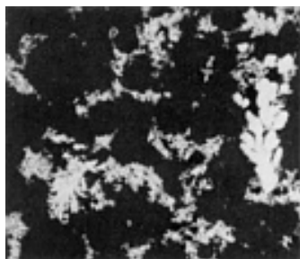
Fig. 13 Electrolytic copper powder showing dendritic structure. 85×. Source: Ref 9
