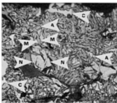
Fig. 143 Nickel steel (Fe-2Ni-0.8C, 6.7 g/cm 3 ). Pressed and sintered (normal processing) in endothermic gas, austenitized 1 h at 870 °C (1600 °F), oil quenched, and tempered 1 h at 260 °C (500 °F). Arrows C indicate carbide particles. Arrows M show a typical martensite platelet, Arrows N surround a nickel-rich region. Arrows A show light-colored regions of retained austenite. Picral. 645×
