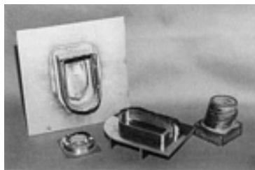
Fig. 12 Thick-walled Ti-6Al-4V laser-based direct fabrication. Source: Ref 41
