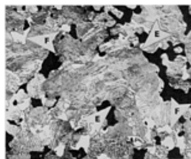
Fig. 55 Atomized iron with 0.8% C ( 6.7 \text{ g/cm}^3 ). See Fig. 53 for processing. P/M steel with 207 MPa (30 ksi) minimum yield strength. Structure is mainly pearlite. Arrows E surround eutectoid (pearlite). Arrows F show a few grains of proeutectoid ferrite. 2% nital. 365 \times
