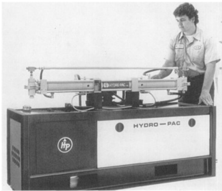
Fig. 6 High-pressure gas compressor. This compressor is rated for operation at 20 MPa (30 ksi) and is powered by a 20 hp electric motor. Courtesy of Hydro-Pac Inc.
