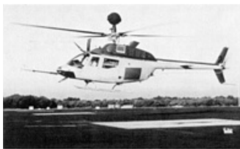
Fig. 4 Mast-mounted sight system (positioned above rotor) using a beryllium optical bench
