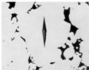
Fig. 8 Knoop indenter mark (100 gf) used as a reference to note the rate of material removal from the surface by measuring the change in length and depth of the indentation. Surrounding black pores in this unetched, pressed and sintered Fe-0.8C alloy ( 6.8 \text{ g/cm}^3 ) are also revealed. 295\times
