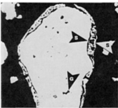
Fig. 153 Ancorsteel 1000 water-atomized, annealed iron. Solid particle with some gas porosity (arrow G) and some surface porosity (arrows S) caused the reduction of oxides picked up during atomization. As-polished. 645×
