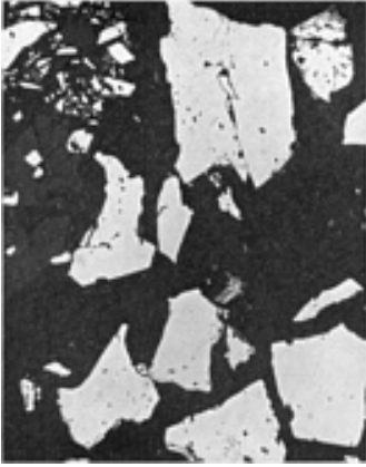
Fig. 1 Cross section of +40 mesh ground magnetite. 30×
