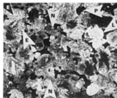
Fig. 100 Same as Fig. 99, but with 0.8% C. Arrows N show nickel-rich areas containing platelets of martensite or bainite. Arrow L indicates a light-etching eutectoid region, and arrow P a pore. Arrows E outline a colony of eutectoid containing thin carbide platelets. 2% nital. 330×
