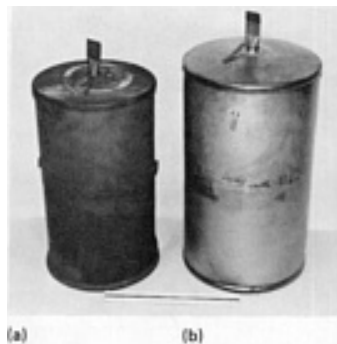
Fig. 10 Cylindrical billet can. (a) After HIP. (b) Before HIP. Source: Ref 22
