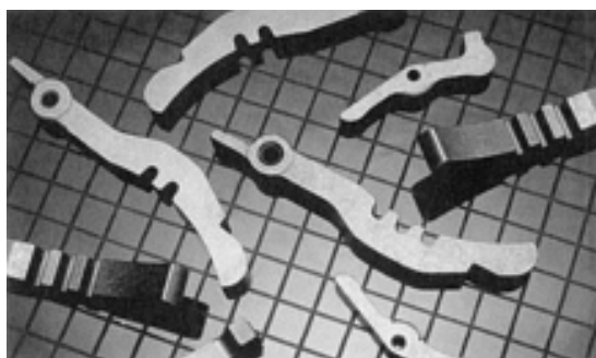
Fig. 28 Steering column tilt levers made from a hybrid P/M alloy (diffusion alloyed FD-0405 material with 2 wt% Ni). Source: Ref 9
