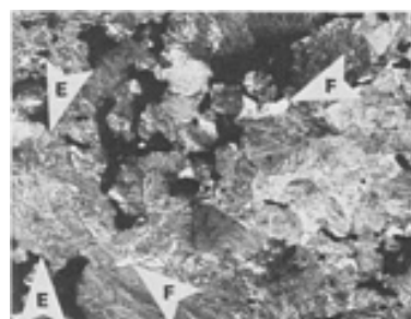
Fig. 56 Atomized iron with 1.0% combined carbon ( 6.7 \text{ g/cm}^3 ). See Fig. 53 for processing. P/M steel with 207 MPa (30 ksi) minimum yield strength. Structure is mainly pearlite. Arrows E surround eutectoid (pearlite). Arrows F show a few grains of proeutectoid ferrite. 2% nital. 310 \times
