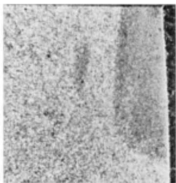
Fig. 11 Ferrous P/M specimen cut without the use of a coolant. Evidence of overheating (dark area at right edge of specimen). Nital. 12×
