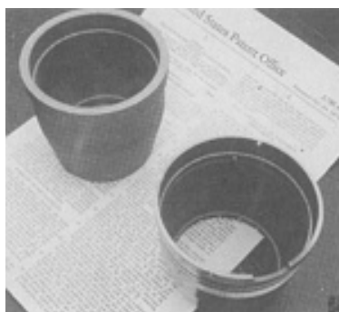
Fig. 5 Sidewinder missile component fabricated by the CHIP process. The left part is the near-net machining preform; the right part is the finished machined component. Courtesy of Dynamet Technology
